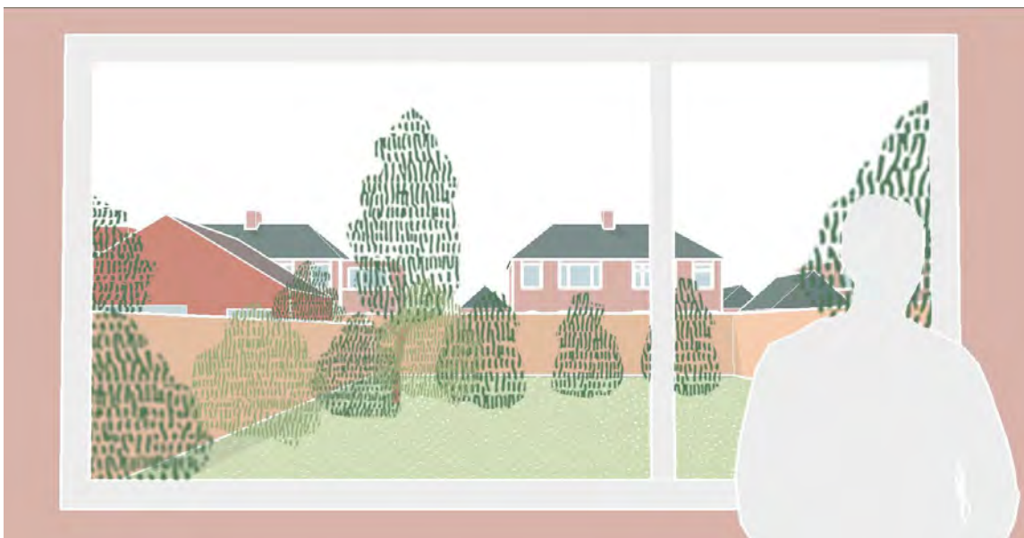
Figure 2.18e: Potential - view from neighbour's kitchen window with a rear garden development built along the boundary. No windows face onto neighbouring garden and proposal drops down towards boundary, to minimise loss of amenity and ensure development potential of neighbouring garden.
