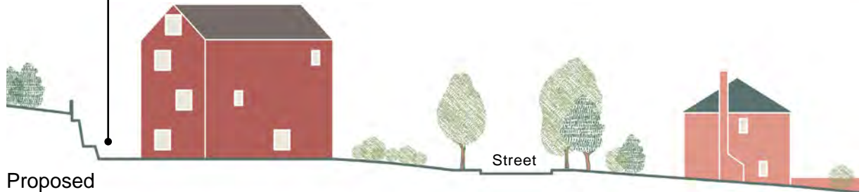
Figure 2.20b: A proposal for redevelopment with semi-submerged ground floor, including lightwell to rear, making use of the topography to provide additional accommodation.
