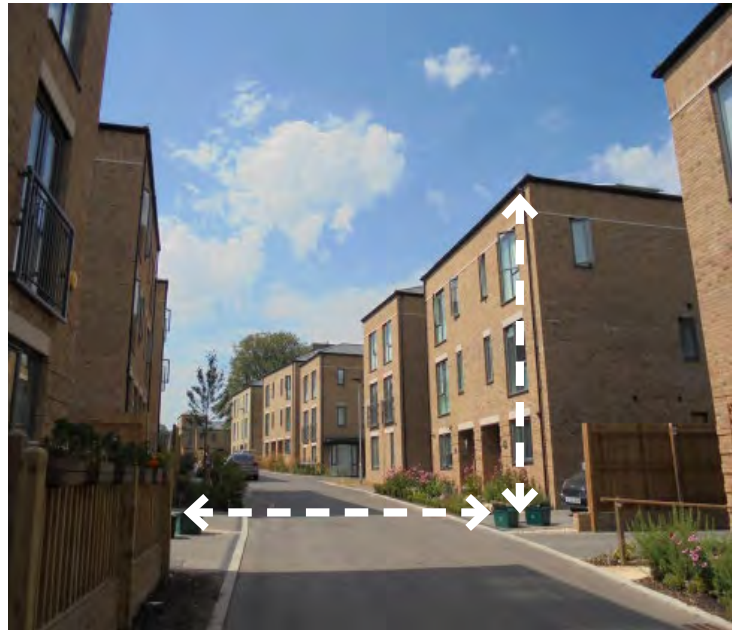
Figure 2.9c: A new suburban street where separation between front elevations is equal to the height of the elevations facing the street.
