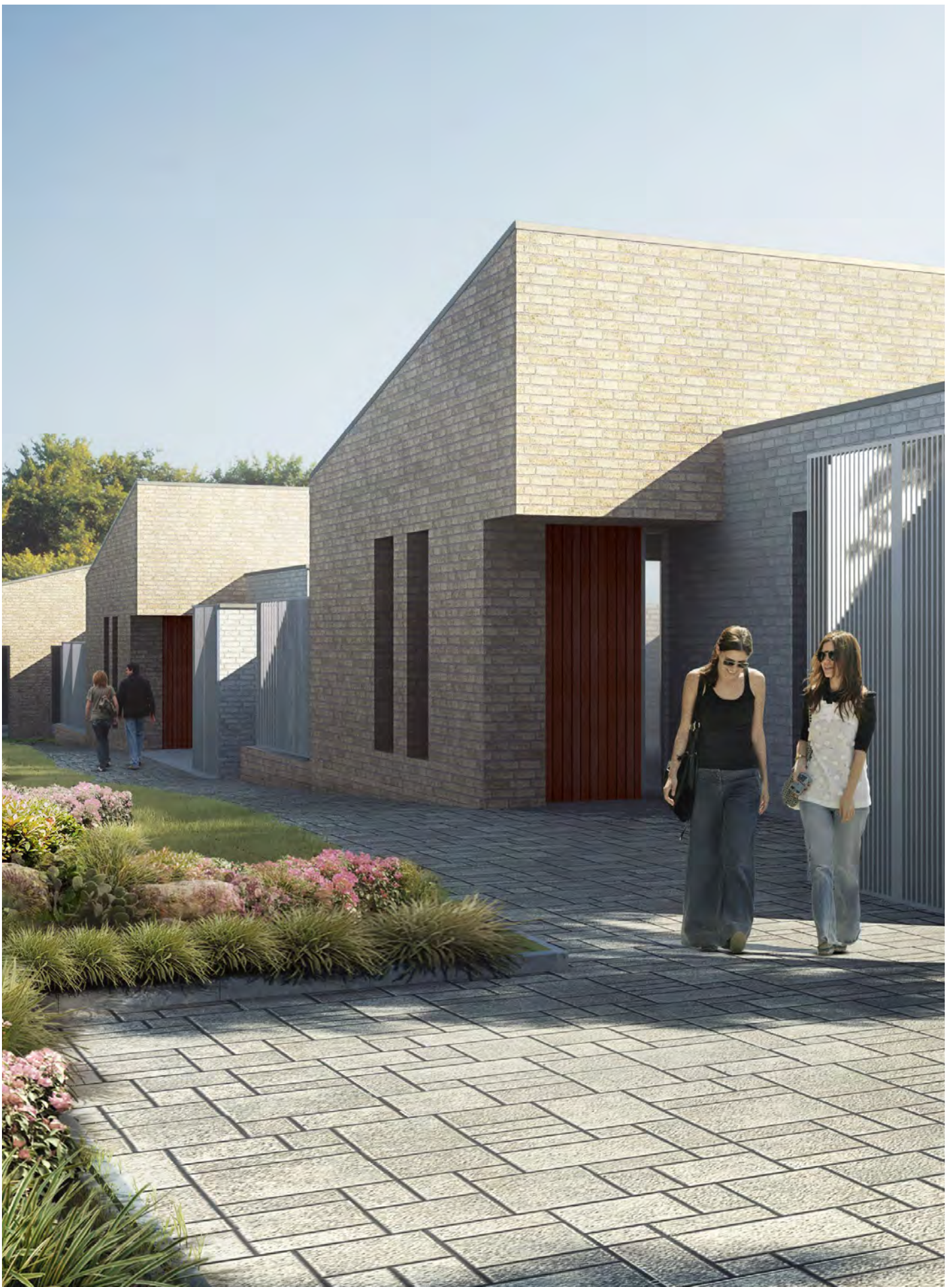
Figure 2.24e: A development of homes in a backland uses a contemporary palette of brick, metal and timber. The most exposed surfaces are made of hardwearing brick, whilst protected features such as doors are made of timber. Refer to guidance 2.21 - 2.23.
