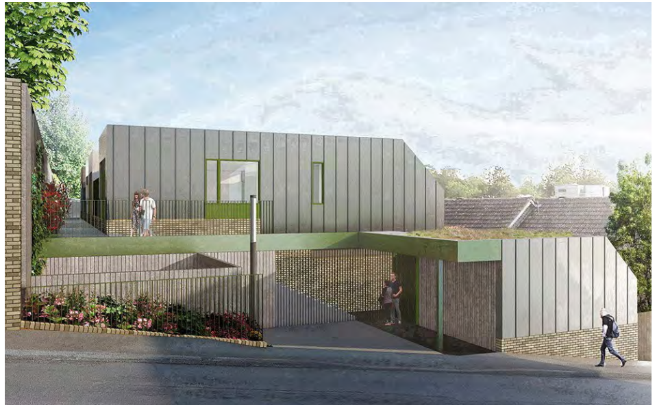
Figure 2.8a: Eagle Hill - example of an Innovative and Original approach designed by Coffey Architects. Use of contemporary form and materials carefully arranged on a back land site (formerly occupied by garages) to create a visual connection with the street. The form is designed to allow residents to look onto their own courtyards rather than out to neighbouring gardens, making use of the sloping site to maximise the delivery of units. Refer section 2.42 for more details on this case study.
