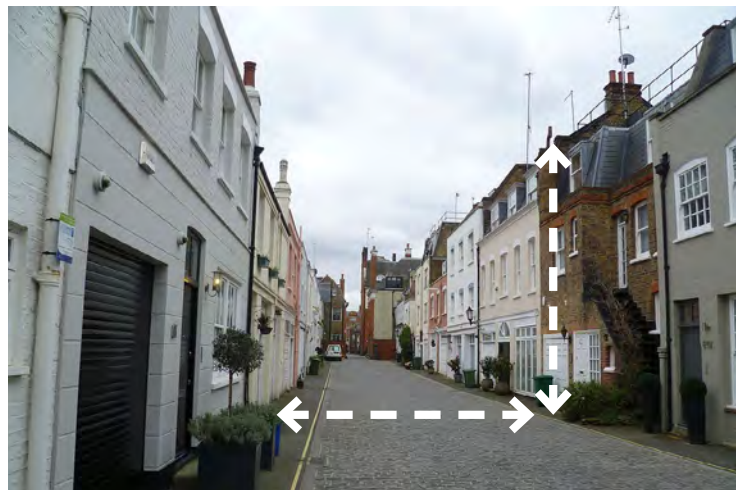
Figure 2.9d: A mews street where separation between front elevations is equal to the height of the elevations facing the street.
